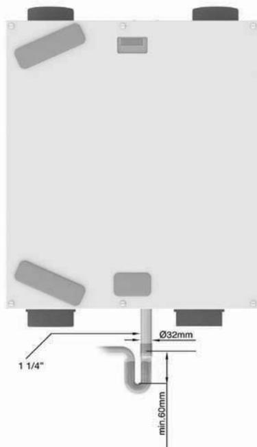
Warm exhaust air is cooled by the outside air in the heat exchanger. This causes the moisture in the indoor air to condense in the heat exchanger. The condensation water created in the heat exchanger is fed to a PVC condensation drain.
