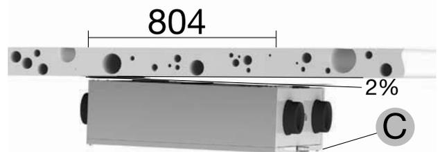
Mount the ComfoAir to a ceiling with a minimum mass of at least 200 kg/m<sup>2</sup>.
