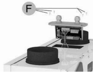
1. Release the electronic cover by unscrewing the 4 screws (F).
